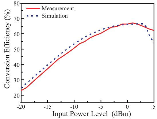
**FIGURE 7.** Measured and simulated RF-DC conversion efficiency versus input power with  $R_L$  of 2.2 kΩ at 2.45 GHz.
