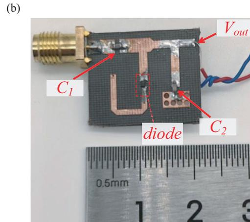
**FIGURE 5.** (a) Layout of the design. (b) Fabricated rectifier.
