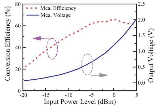
**FIGURE 9.** Measured conversion efficiency of the rectenna.
